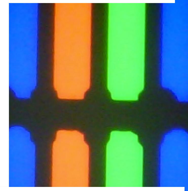
$$Magnification \ M = \frac{Number \ of \ Screen \ Pixels \times Size \ Screen \ Pixels}{Size \ of \ Webcam \ picture}$$
